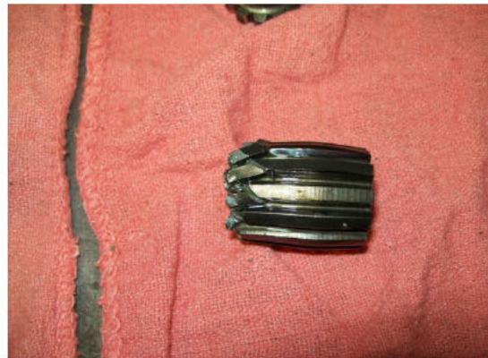
Figure 36: Fractured splined drive
