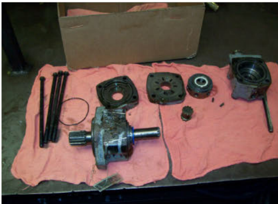
Figure 35: Fractured splined drive
