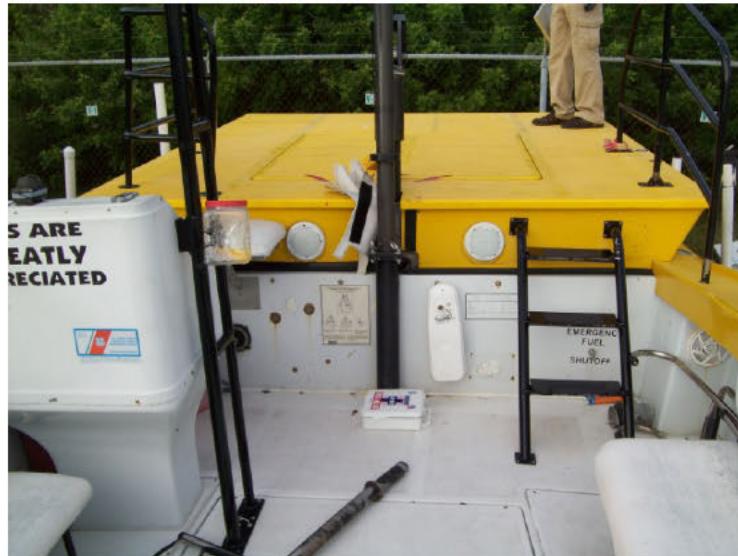
Figure 2: SKY SCREAMER landing platform and tow post.
