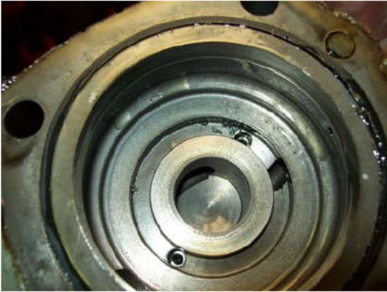
Figure 31: Metal fragments within valve housing
