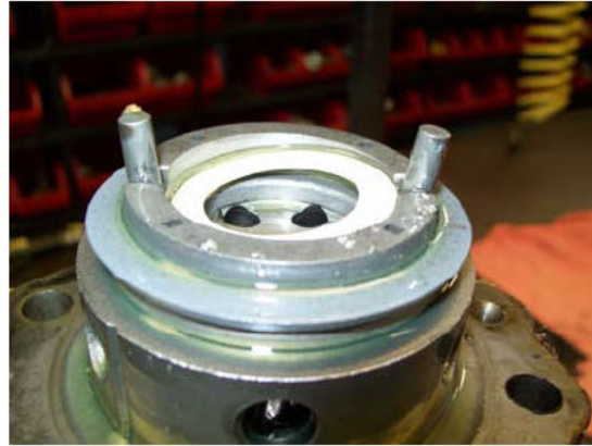
Figure 32: Metal fragments on outer face seal and valve assembly
