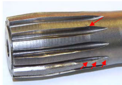
Figure 39: Secondary cracking on splined drive that inserts into bearing housing
