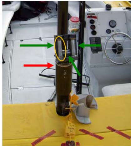
Figure 47: Tow post / roller head assembly
