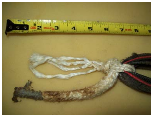
Figure 46: Parted towline at yoke
