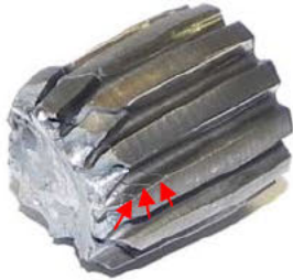
Figure 38: Secondary cracking to geroler side of splined drive
