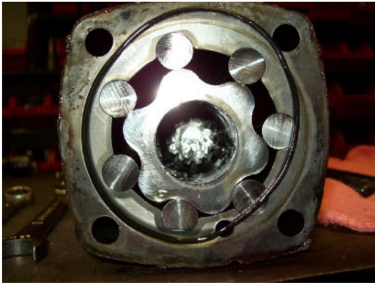
Figure 33: Fractured splined drive stuck inside of geroler assembly
