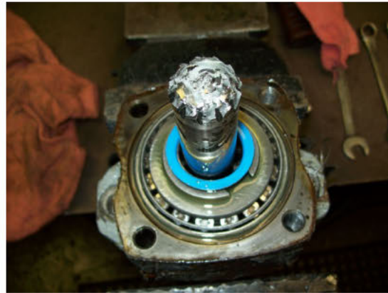
Figure 34: Fractured splined drive
